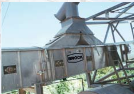
2-way inlet for Brock's reversing conveyor configuration
