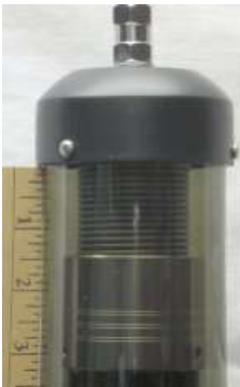
Model 100A-HP -- 14.2 MHz with 5 ft. whip @ 1 1/2" of coil showing
