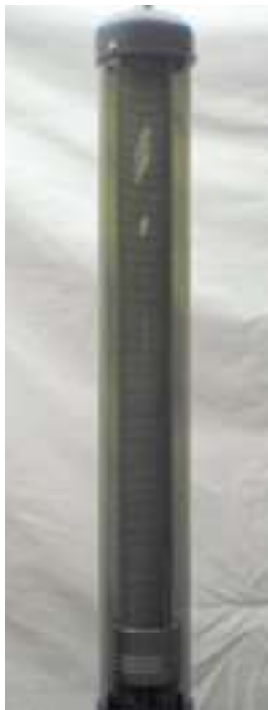
Model 100A-HP -- 3.5 MHz with 5 ft. whip @ 18" of coil showing
