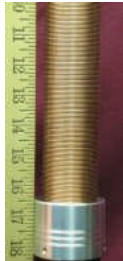
Model 300A -- 1.8 MHz with 5 ft. whip and 16 1/2" of coil showing
