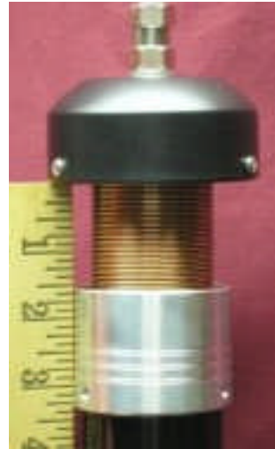
Model 400 -- 7.1 MHz with 5 ft. whip and 1 1/2" of coil showing
