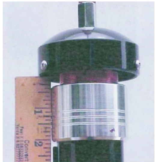
Model 75A "Stubby" -- 14.2 MHz with 5 ft. whip @ 1/2" of coil showing
