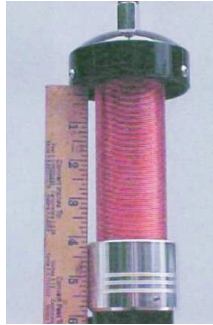
Model 75A "Stubby" -- 3.9 MHz with 5 ft. whip @ 4" of coil showing
