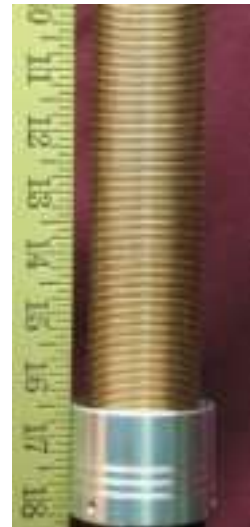
Model 400 -- 1.8 MHz with 5 ft. whip and 16 1/2" of coil showing
