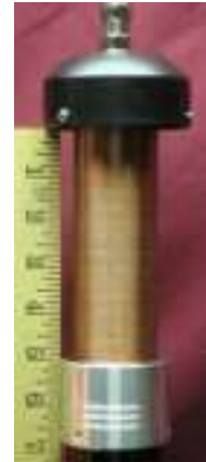
Model 400 -- 3.5 MHz with 5 ft. whip with 5" of coil showing
