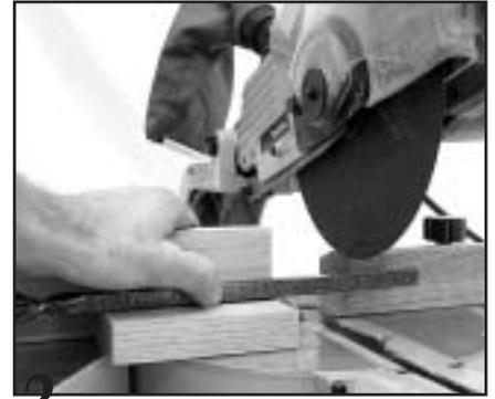
**3.** After adding  $5/8''$  for insertion into the rail and  $3/4''$  for insertion into the tread (a total of  $1-3/8''$ ), use a chop saw equipped with a standard  $1/8''$  flexible cut-off blade to trim the baluster to the exact length.
