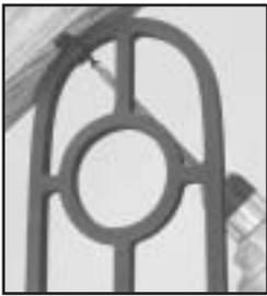
C-2932 Arch Medallion Balusters are shipped with installation brackets and hardware included. After installing the baluster into the treads, attach to rail by predrilling and screwing the brackets into place.
