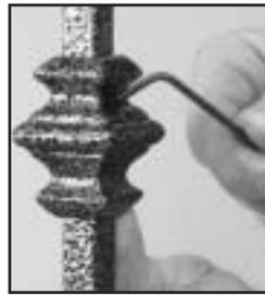
The Adjustable Collar, when used with the C-2555 straight forged baluster, can be used to design a distinctive pattern within any forged system. Place the required number of adjustable collars on each C-2555 straight baluster before installing. After the balusters are installed, use an allen wrench to tighten the collar's set screw, permanently attaching the collar at the desired location.
